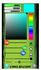
Click the Power Button (bottom right) to active the lights. This is your Basic mode. Move the bar to adjust the color. Adjust the brightness of any color. Can also flash or breathe on any color. Use the Interval bar to change the speed.
