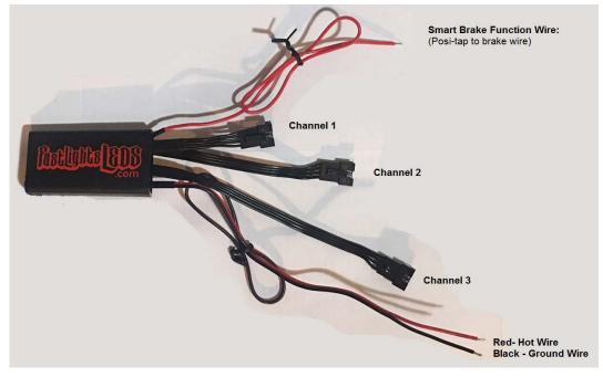
• Connect the Hot and the Ground to the battery using your inline fuse provided.
